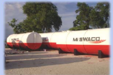
Drilling Fluid Storage Tanks
